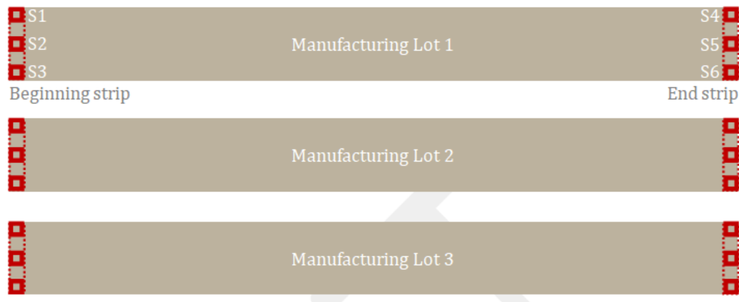
Figure 5.1.1.1a: Locations of test strips and material samples.
