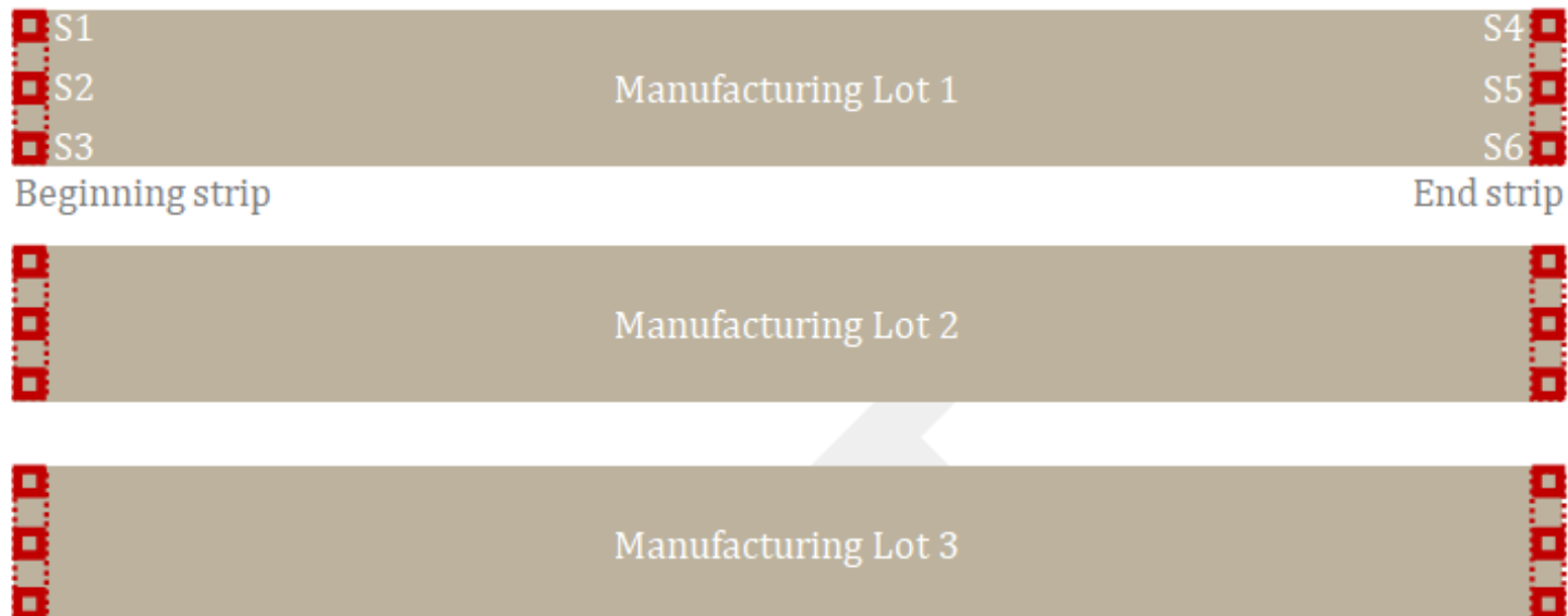
Figure 5.1.1.1a: Locations of test strips and material samples.
