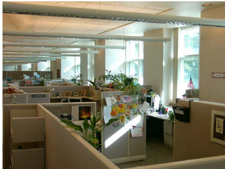
Figure 6: Luminaire arrangement on top floor of CSC building with skylights Note luminaires perpendicular to windows, top floors only.
