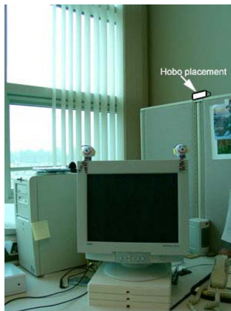
Figure 27: Hobo placement on a partition.
