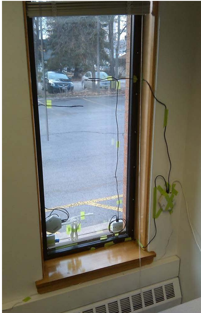
Figure 7. Instrumented window (following retrofit) with data loggers between the original glass layer and the Hi-R panel, as well as on the room side of the glass, frame, and wall
