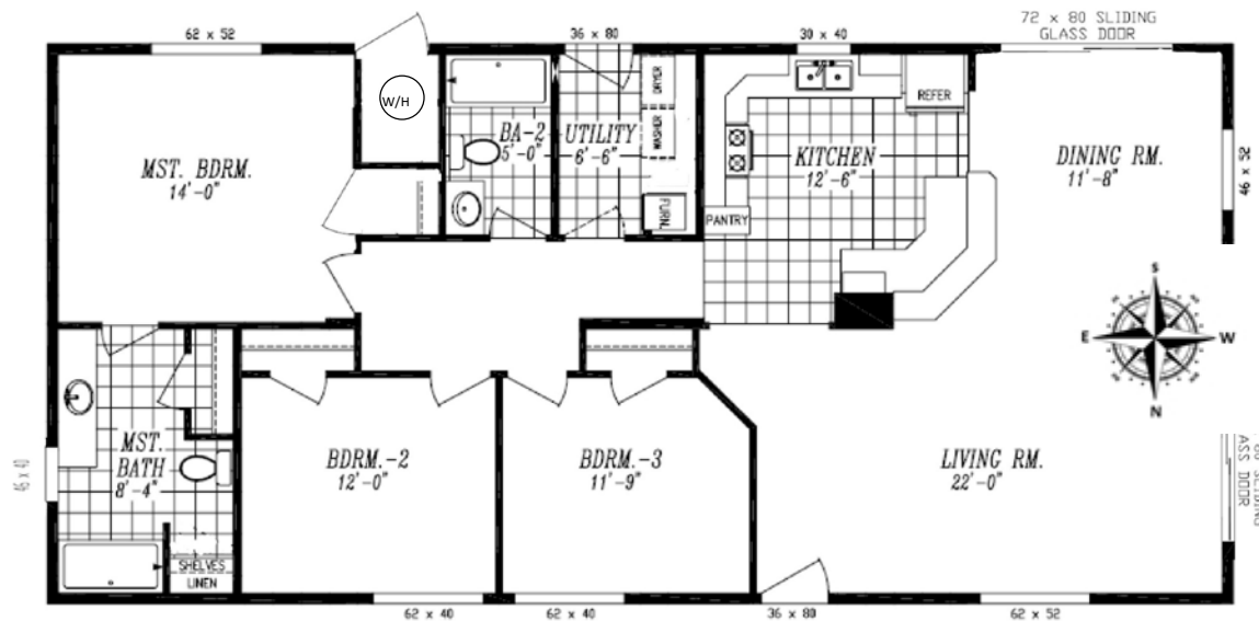
Figure 3.1. Floor Plan of the Lab Homes as Constructed
