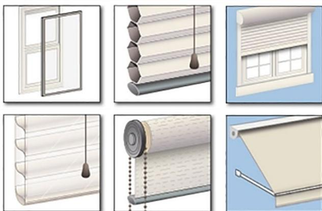
Starting from top left: storm window, cellular shade, exterior roller shutter, sheer shade, roller shade, and retractable awning.
