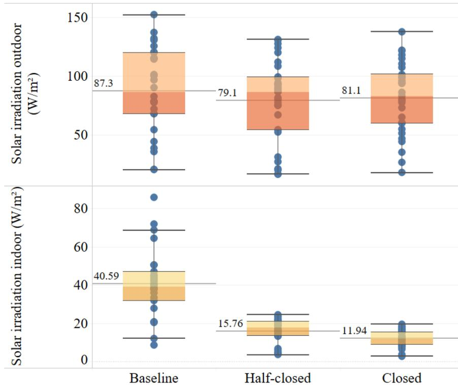
**Figure 8. Distribution of daily average (data from 8:00 a.m. to 7:00 p.m.) of outdoor and transmitted solar irradiation for different cases.**
