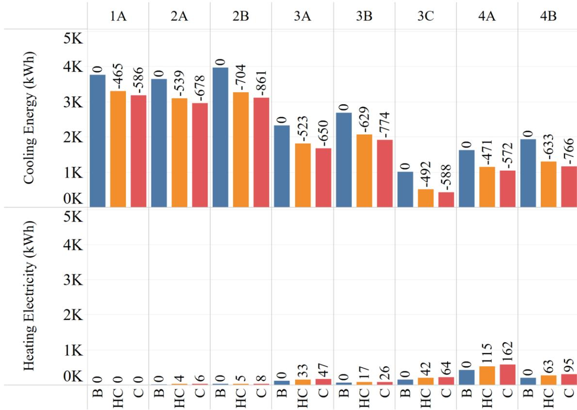
Figure A.1. Heating and cooling energy consumption for residential prototype buildings
