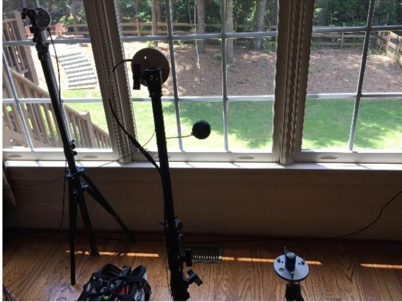
**Figure 5. Illuminance sensors on the building interior.**
