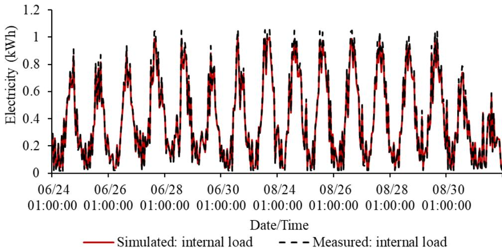
Figure 12. Measured and simulated internal load for the test house.
