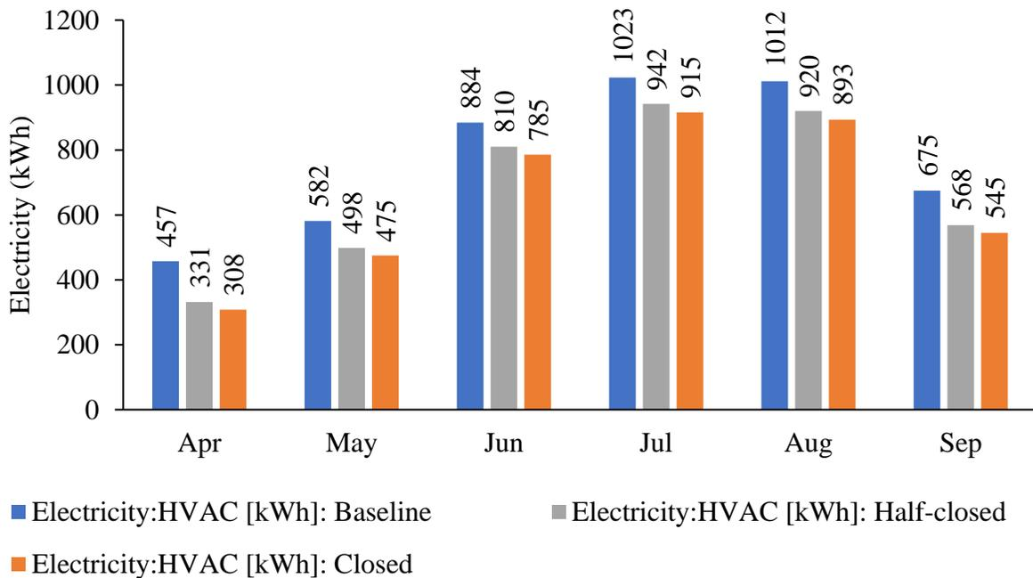
**Figure 14. Monthly HVAC electricity from the test house model simulation for April through September.**
