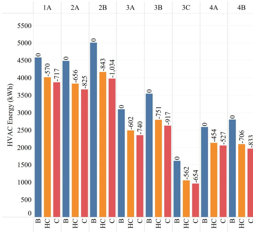
Figure 15. HVAC energy consumption for prototype buildings at six different climate locations for eight different cases. (B = baseline; C = closed; HC = half closed).
