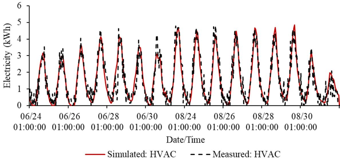
**Figure 13. Measured and simulated HVAC consumption for the baseline case.**
