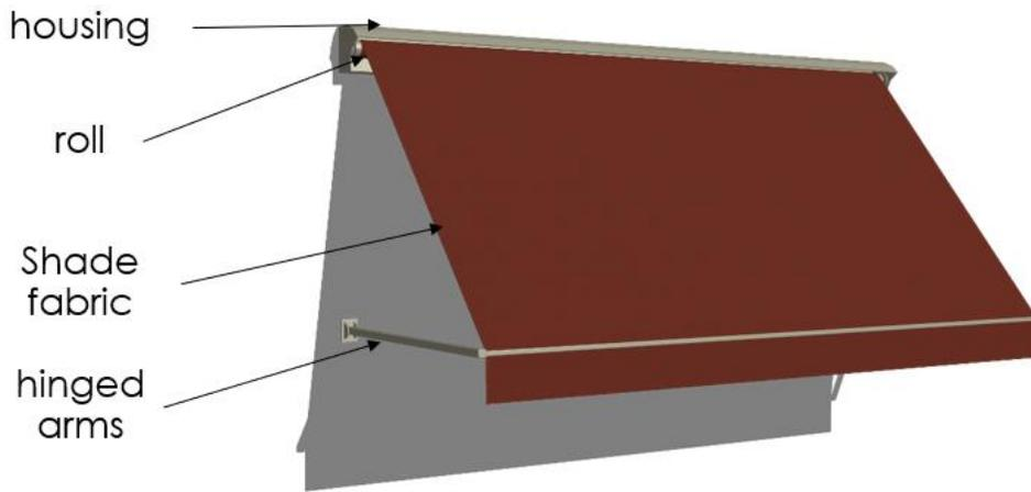
Figure 1. A sketch of a drop-arm awning system.
