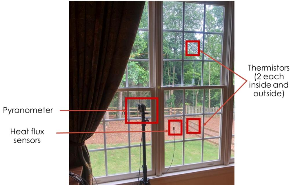
**Figure 3. Placement of various sensors installed on one window.**
