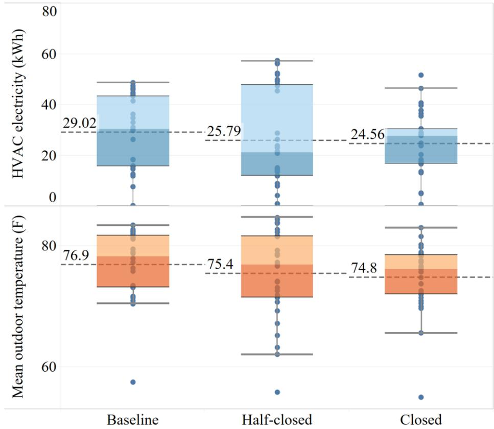
Figure 10. Box plot of daily energy consumption and corresponding outdoor temperature for three cases.
