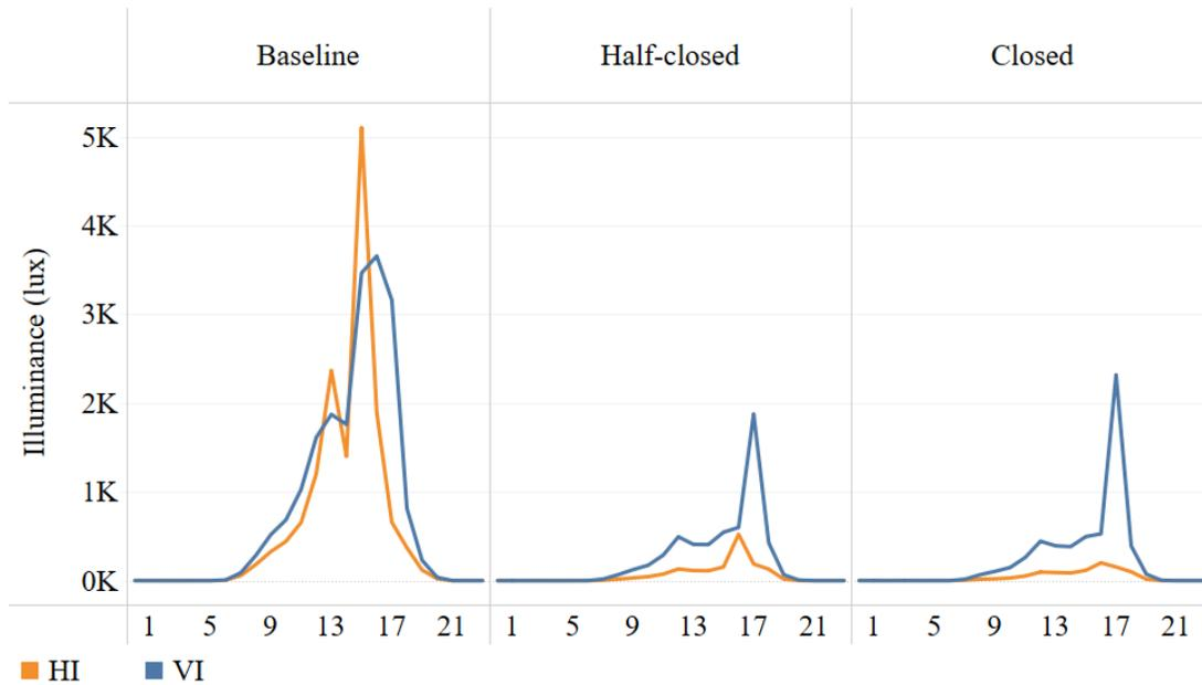
Figure 9. Average VI and HI for different test cases at each hour of the day.
