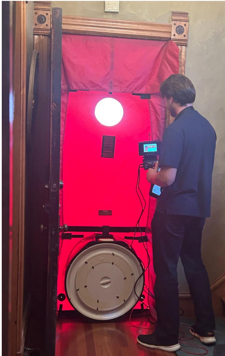
Figure 7. Example of a blower door test.
